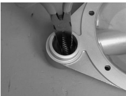
Remove the valve stops [3] and the ball valves [15] out of the side housings [1]. For the AD 32 and AD 50 the use of a screwdriver to remove the valve stops maybe is more convenient.
