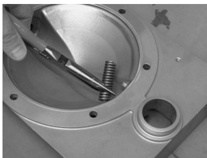
Remove the valve stops [3] and the ball valves [15] out of the side housings [1]. For the AD 32 and AD 50 the use of a screwdriver to remove the valve stops maybe is more convenient.
