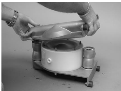
Remove side housing [1] and suction/discharge ports [2].
