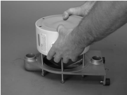
Remove the center block [16] by gently pulling apart.
