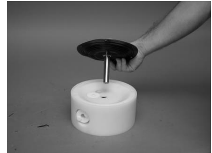
Pull the other diaphragm [14] together with the shaft [13] out of the center block [16].
