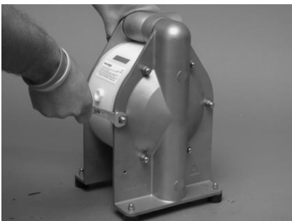
Loosen nuts of the housing bolts on one side of the pump.
