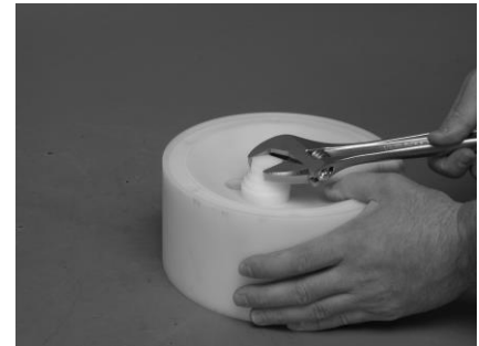
To remove the PERSWING P air control system, screw off both end caps using the plastic mounting tool delivered with the pump. Take out main and pilot piston.
