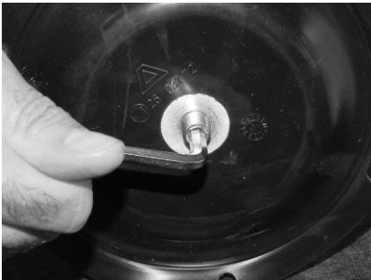
Screw out the set screws, shaft [13a].
