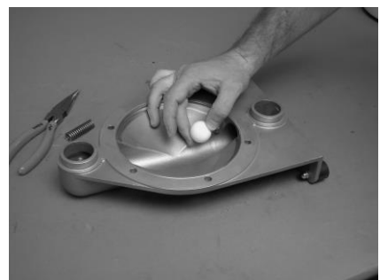
Remove the valve stops [3] and the ball valves [15] out of the side housings [1]. For the AD 32 and AD 50 the use of a screwdriver to remove the valve stops maybe is more convenient.
