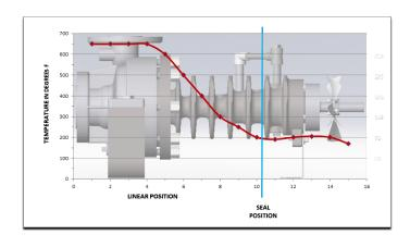
The air fan-cooled design of RA series pumps permits temperature drop in the pump from the casing to seal faces. When pumping at 650° (343°C), the seal face temperature is 200°F (93°C). The efficient gradient breakdown protects the mechanical seal and bearing.
