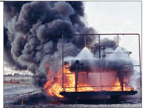
N6 nozzles protect a propane storage tank from fire and explosion.
