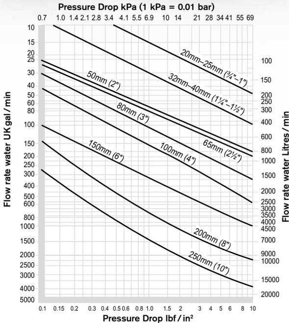
A single basket OV filter is required to protect pipeline equipment to a level of 200 microns. The media is water at 20°C, at a pressure of 4 bar g and having a flow rate of 600 litres/min. A clean basket pressure drop of no more than 34 kPa is acceptable.
