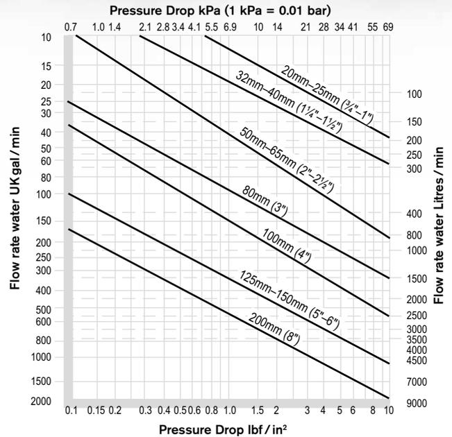
A dual basket OW filter is required to filter particles the size of 80 microns from lubricating oil which has a viscosity of 230 centistokes at 40°C. The flowrate of oil is 150 litres/min at a pressure of 10 bar g. A clean basket pressure drop of no more than 41 kPa is acceptable.
