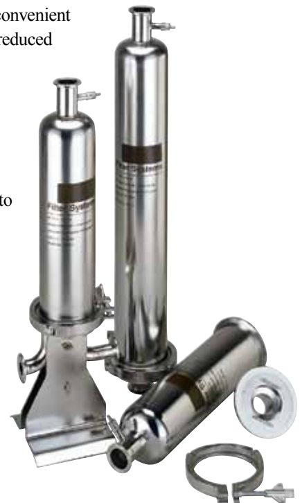
Figure 15 – 3M Purification manufactures a wide range of sanitary design, pre and final filter housings. The ZMS/ZVS models (shown above) accommodate a single 10" - 40" filter cartridge while the ZWC/ZWB models (not shown) accommodate up to 21 10" - 40" cartridges.
