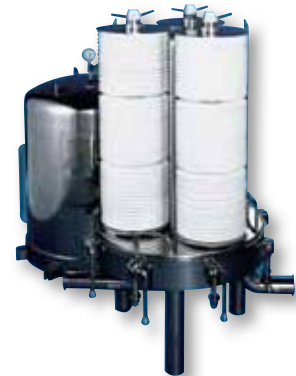
Figure 18 – Like all Zeta Plus™ housings, this 12ZP9 utilizes an easy to operate, spring loaded sealing system (seen at the top of each filter stack) to ensure reliable cartridge to housing sealing. The housing contains 9 Zeta Plus cartridges and is capable of service flow rates up to 45 GPM (90 HL/hr).
