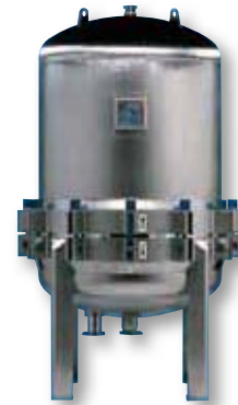
Figure 17. – This 12ZP48 housing contains 48 Zeta Plus™ cartridges and is capable of service flow rates up to 240 GPM (480 HL/hr).
