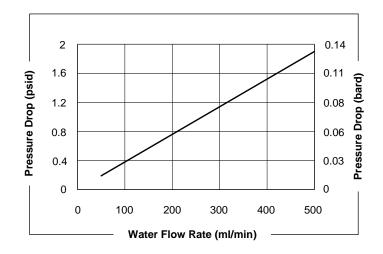
Curves represent nominal values, generated using water on the Lumenside at 20° C with 50 torr of vacuum drawn on both Shellside ports. The estimated vacuum volume guideline is based on a flow rate at 20° C, 50 Torr. Characteristics may change under different operating conditions.
