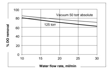
Curves represent nominal values generated using water on the shellside and vacuum on the lumenside at 20° C. Characteristics may change under different operating conditions.
