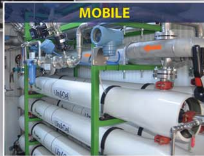
8x80-inch Mobile Deoxygenation System in Refinery
