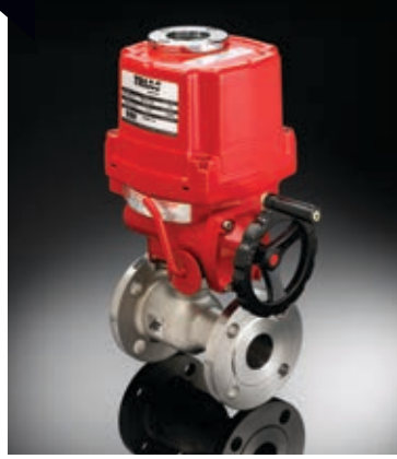
150# Flanged Firesafe tested to API-607
