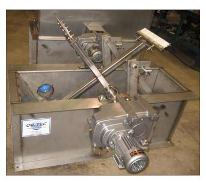
A simple self-cleaning screen for MBR systems municpal industrial effluents, sewage works, recirculation waters, feedwaters, etc.
