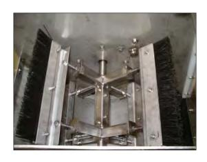
Slowly rotating brushes remove screened particles and a dampened scraper system discharges them from the screen ready for disposal
