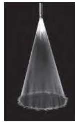
SPRAY PATTERN 30° hollow cone
