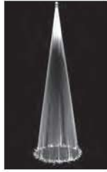
SPRAY PATTERN 15° hollow cone
