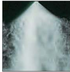
SPRAY PATTERN fine fog droplets
