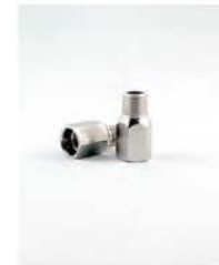
M10FSS THREAD ADAPTER 1/8 npt female to 10mm x 0.75 male stainless steel
