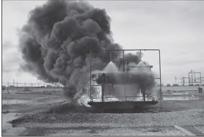
#210 NOZZLES PROTECT A PROPANE STORAGE TANK FROM FIRE & EXPLOSION
