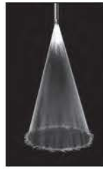
SPRAY PATTERN 30° hollow cone
