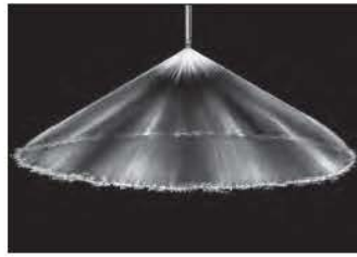
SPRAY PATTERN 120° hollow cone
