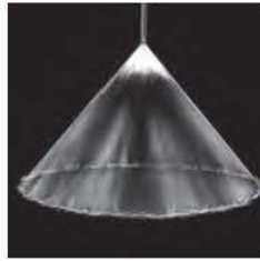
SPRAY PATTERN medium angle - hollow cone
