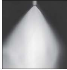
SPRAY PATTERN fine fog droplets
