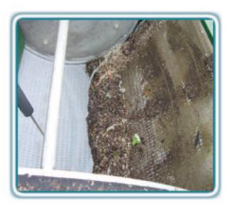
The MYCO media filter is a fully automatic system that ensures efficient cleaning of any process fluid while optimizing the amount of media used. The solids are discharged as a cake for easy handling and disposal.
