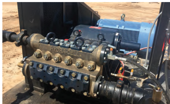
Hydra-Cell features a seal-less design that separates the liquid end from the hydraulic end. This enables the pump to tolerate solids, abrasives, and particulates, handle non-lubricating fluids, and run dry without damage to the pump.
